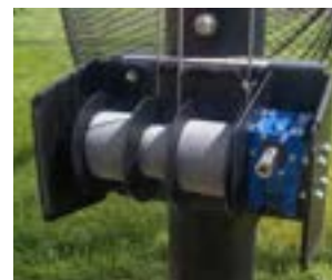
Winch and cable designed for single-person operation
