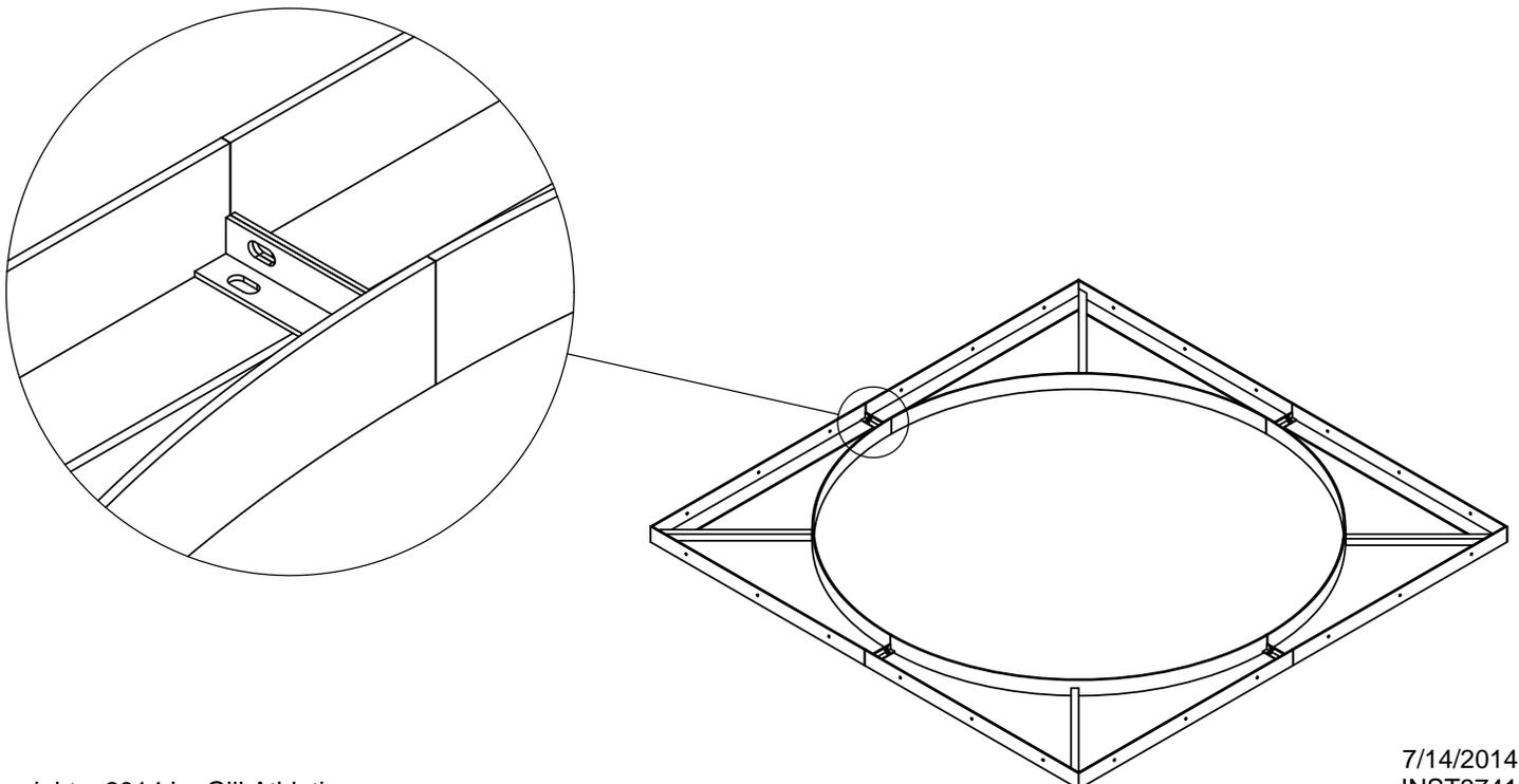
6) Outer pour should be flush and level with exterior edge, or to the required level for an artificial surface. Inner pour should be level, 3/4" from the top edge of the frame.
