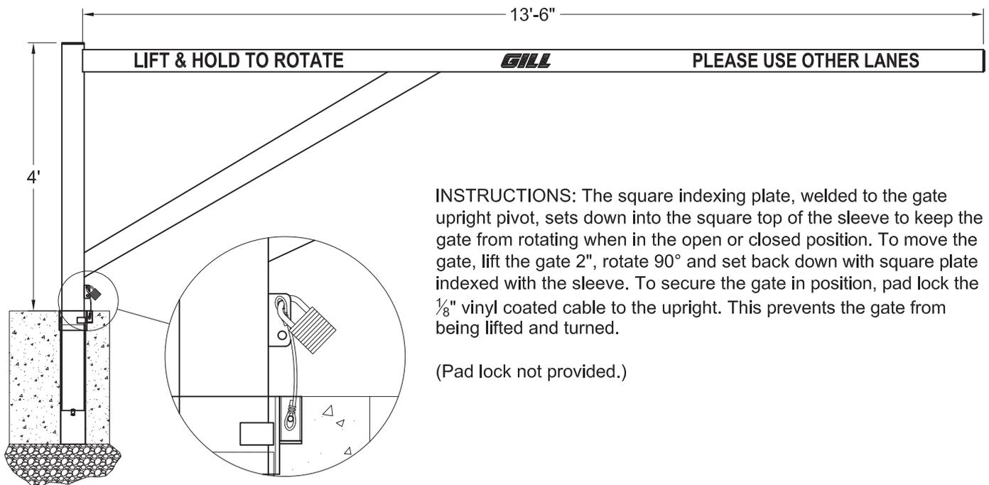
**INSTRUCTIONS:** The square indexing plate, welded to the gate upright pivot, sets down into the square top of the sleeve to keep the gate from rotating when in the open or closed position. To move the gate, lift the gate 2", rotate 90° and set back down with square plate indexed with the sleeve. To secure the gate in position, pad lock the 1/8" vinyl coated cable to the upright. This prevents the gate from being lifted and turned.
