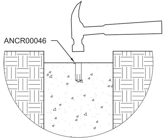
Use the installation tool and a hammer to set anchor.
