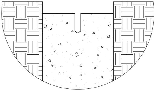
With the threaded opening pointing up, insert the anchor into the hole.
