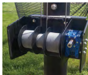
Winch and cable designed for single-person operation
